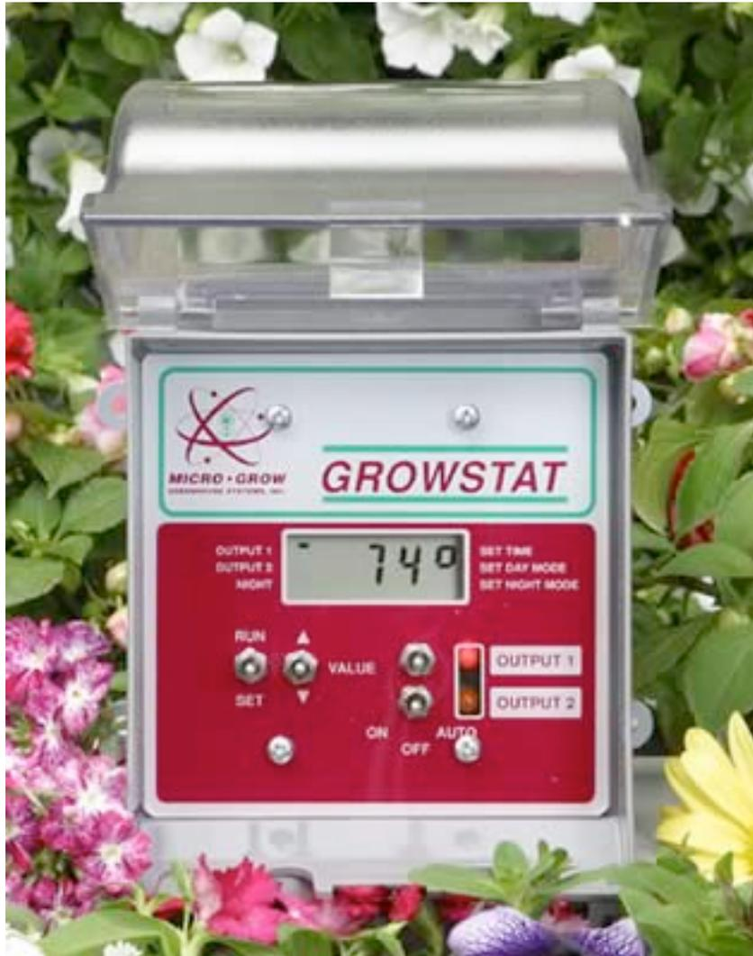
Exact control of individual heating or cooling needs. Will operate one stage of heating and cooling in a single zone, or two stages of either in a single zone. Fogging control version available using precise sensors for humidity, temperature, or both.
